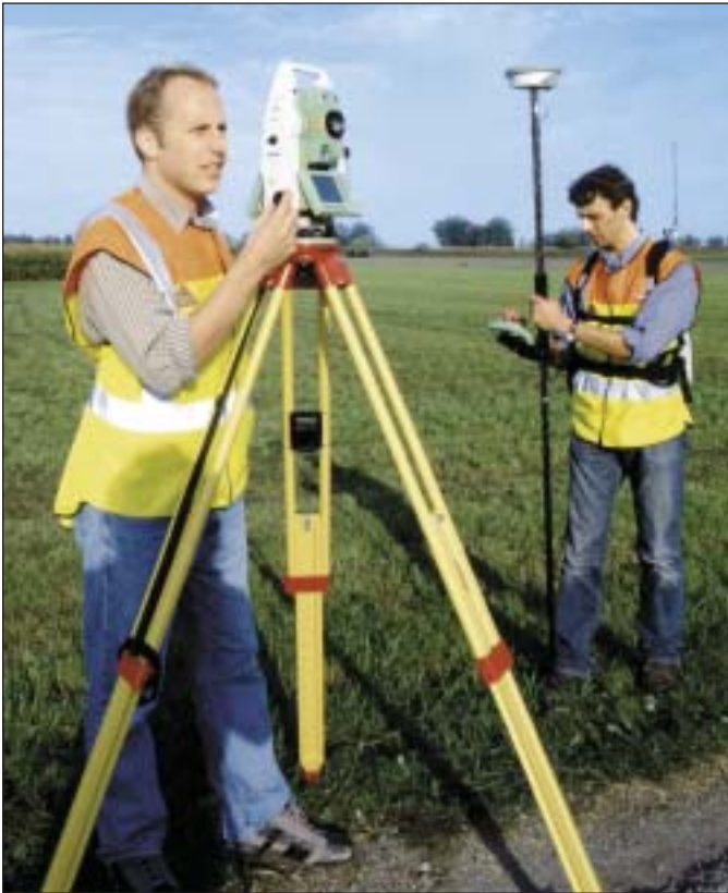
Having positioned the SmartStation, the Smart Antenna is removed and transformed into an RTK rover.
